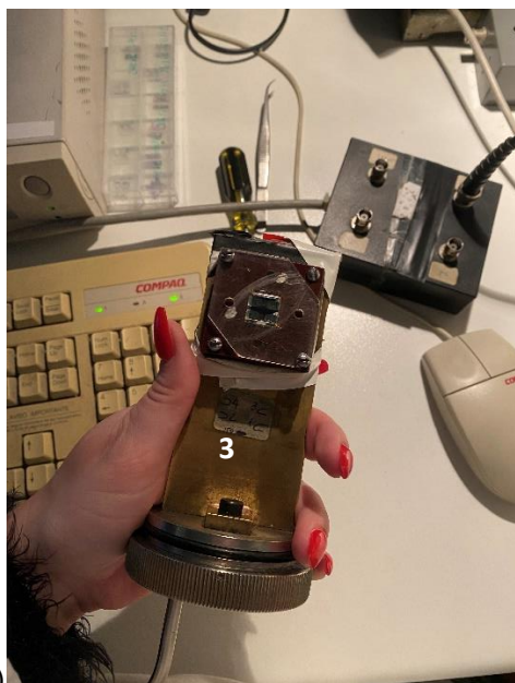
Figure 2.4 a) Complete home-made set up and b) Support with contacts for the OLED for dark analysis
