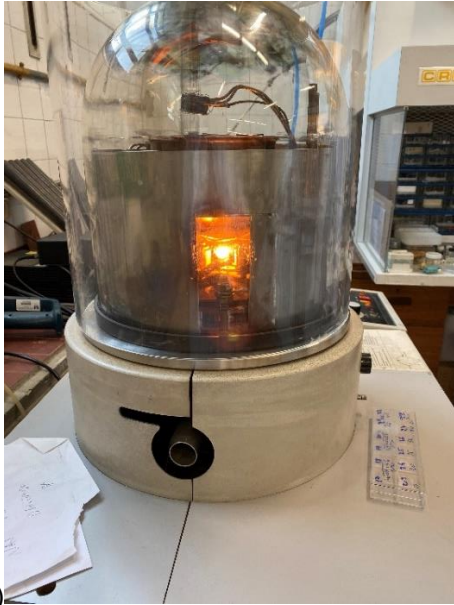
Figure 2.5 a) Top view of spaced 4 gold stripes deposited by thermal evaporator and b) Gold during evaporation
